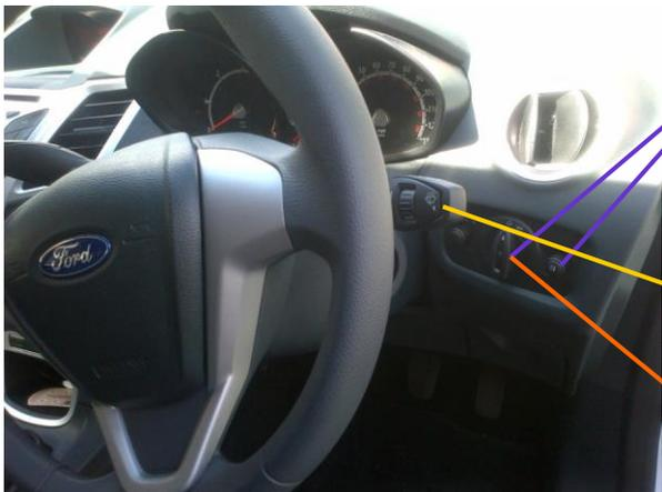
To turn on fog lights turn on the dipped headlights then press the fog light button alongside
