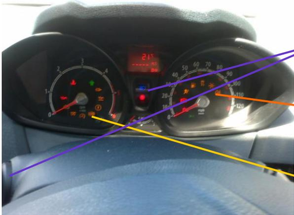
Blue light is on when main beam is turned on
